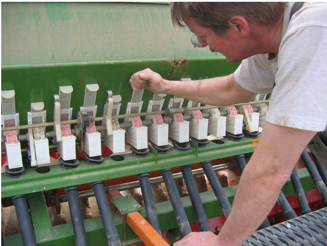
Fig. 5.1.5: Sparsely sown areas or strips are created during the sowing of cereal crops by closing individual coulters of the seed drill. Picture: R. Oppermann.
