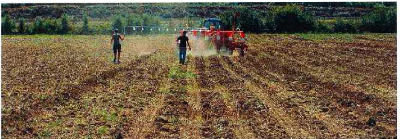
Experimental group C: the bar that supports the 10 cages is kept at 1.8 m height by two operators. They proceed at 4 m from the seeder, laterally, so as to intercept the dust cloud shifted by the wind.
