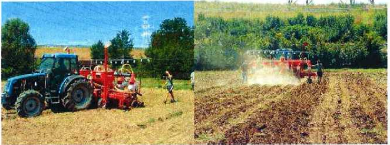
Experimental group A: the horizontal bar which supports the 10 cages at 2.5 m height is fixed to the posterior part of the seeder. The picture on the right shows the system during the seeding.
