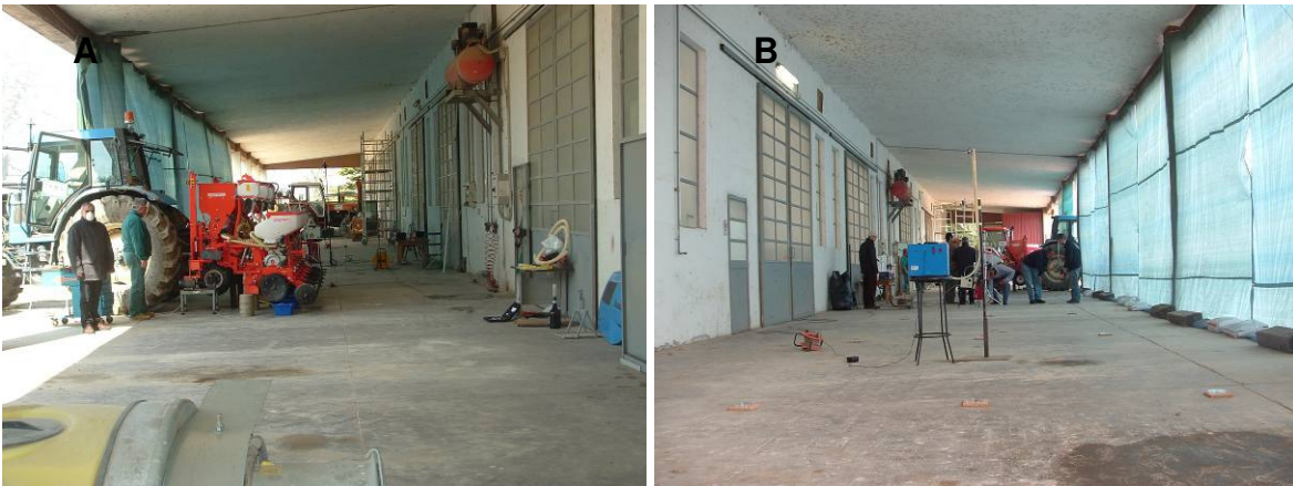
Figure 4 – Fixed point test zone. A) visualization of the seeder raised off the ground , and in the lower left-hand corner the atomizer utilized for wind generation; B) View from the opposite end of the portico, showing the Petri dishes placed on the ground and the air samplers at the various distances.
