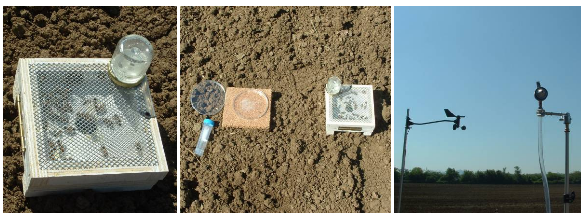
Figure 9 – From the left: cage with feeder dispenser, containing roughly 30 bees; small cage on the ground beside a Petri dish during one of the sowing trials; anemometer recording wind speed and direction, and air sampler capsule containing the filter.
