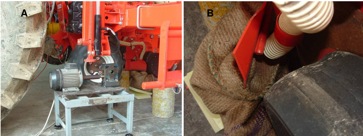
Figure 2 – A) Electric motor to start up and drive the seeding device from stationary with the machine raised off the ground; B) a container lined with a wet jute sack was placed beneath the coulter in order to protect the dust against turbulence, simulating real field conditions.
