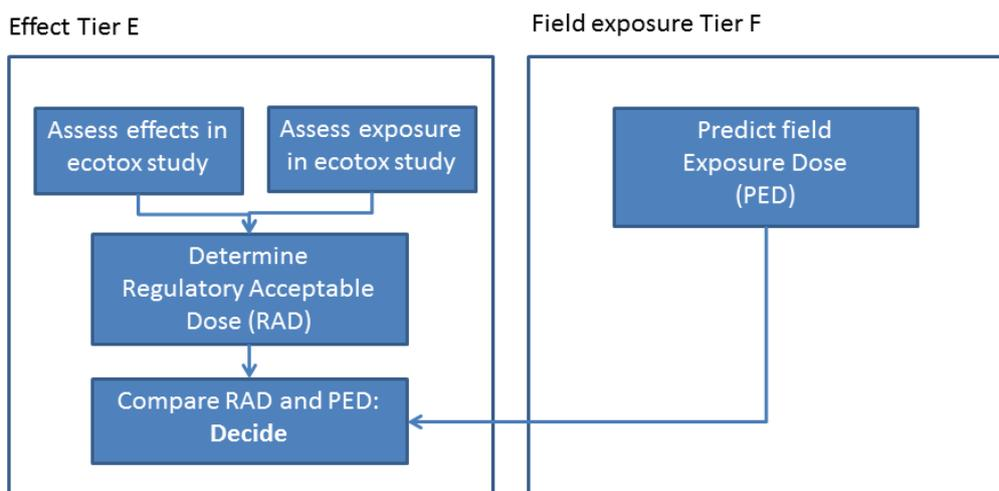
**Figure 18:** Schematic representation of the two types of exposure assessments which are needed in any combination of tiers of the effect and field-exposure flow charts (adapted from Boesten et al., 2007)
