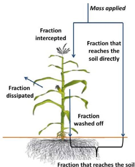
**Figure 23:** Schematic overview of the processes occurring at the crop canopy. The fraction of the dose reaching the soil is the sum of wash-off from the canopy and the fraction of the dose that reaches the soil directly
